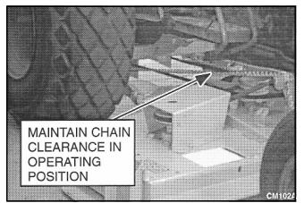
Figure 2. Chain Clearance from Drive Belt
